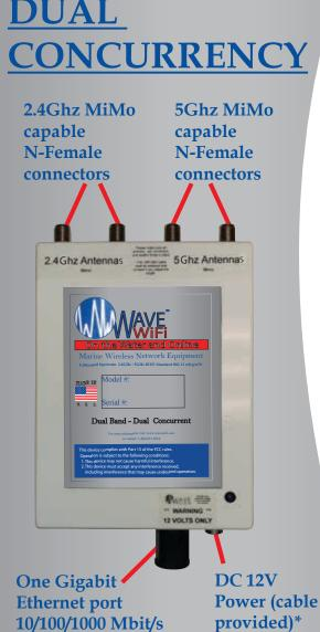
MODEL EC HP DUAL BAND (DB) CPU 600Mhz ETHERNET One Gigabit port 10/100/1000 Mbit/s Fast Ethernet port 802.11 b/g/n 2.4Ghz 2400MHz - 2500MHz WIRELESS 802.11 a/n 5Ghz 802.11 a/n 5Ghz (5Ghz ac optional) Freq. Range 4920 - 5920 MHz | Freq. Range 4920 - 6100\* MHz DC 12V Power cable POWER **OPERATING** -22F to +140F / -33C to +60C TEMP. CONNECTOR Four N-Female Antenna connectors (two 2.4Ghz) + (two 5Ghz)
