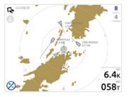
**Intelligent target filtering**: Reduces screen clutter showing only those vessels with a collision risk.
