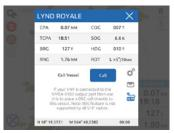
**DSC calls:** Place calls directly to a vessel by touching it on the screen. (Works with ICOM VHF radios)
