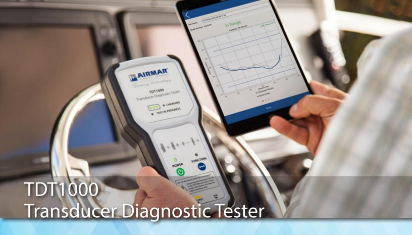
Eliminate the guesswork and determine if a transducer is in proper working condition quickly with AIRMAR's TDT1000, the first transducer diagnostic test device for use with most transducers. Connect directly to AIRMAR's database via the SensorCheck™ App and compare the transducer onboard the vessel to its original, factory-approved test results.
