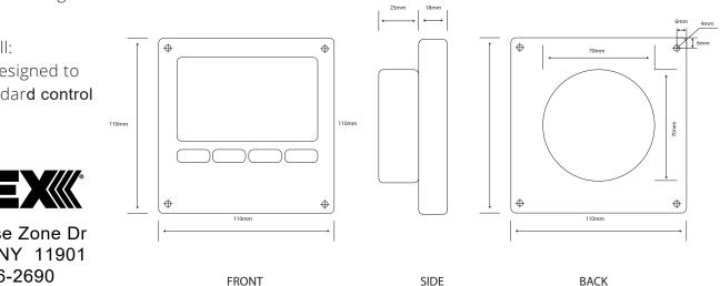
Easy to install: SP110C is designed to 110mm standard control head size.
