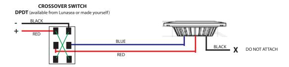
Using three wire setup apply power to either of the + leads - HI/LO or White/Red(Blue) capability
