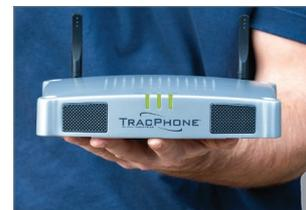
The VSAT-Hub is the TracPhone V30's ultra-compact belowdecks unit that eliminates the need for rack mounting. Coupled with the compact digital
