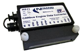
The RS11 Engine Data Converter converts tachometer signals and analog gauge voltages from virtually any engine into CANbus digital messages (J-1939, NMEA 2000). It is configurable for either single or dual engine installations and includes a USB PC interface for initial configuration, data monitoring, and software updates. Output messages are applied to the CANbus for display by compatible devices.
