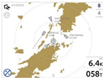
**Intelligent target filtering:** Reduces screen clutter showing only those vessels with a collision risk.
