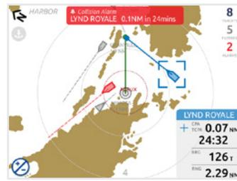
**Alarm banner:** Highlights the most critical alarm while also sounding an audible alarm.
