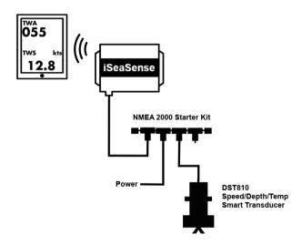
Basic cabling kit includes spare NMEA 2000 port and 1m connect cable for 3<sup>rd</sup> party display or device
