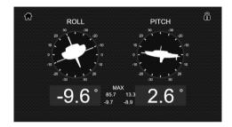
Graphic displays of boat heel and pitch with recorded maximum values. The boat heel data can be used for precision speed calibration – ideal for racing and accurate TWS/TWA and VMG data
