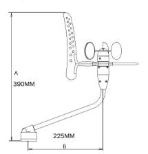
WND200 Pack includes mast head unit, 20m cable and NMEA 2000 interface. Included as standard in Pack 2
