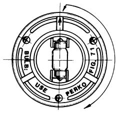
NOTE: ARROW MOLDED INTO PLASTIC BASE TO INDICATE BULB POSITION
