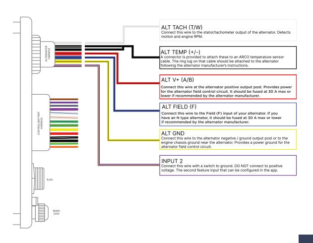
Follow your alternator wiring harness connections carefully. The wiring harness instructions are included within this manual and can also be enlarged in the app by long pressing the wiring harness instruction image.
