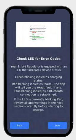
There is an LED light near the ports on your regulator. If the LED is currently blinking red, review all of the app warnings in the next section.
