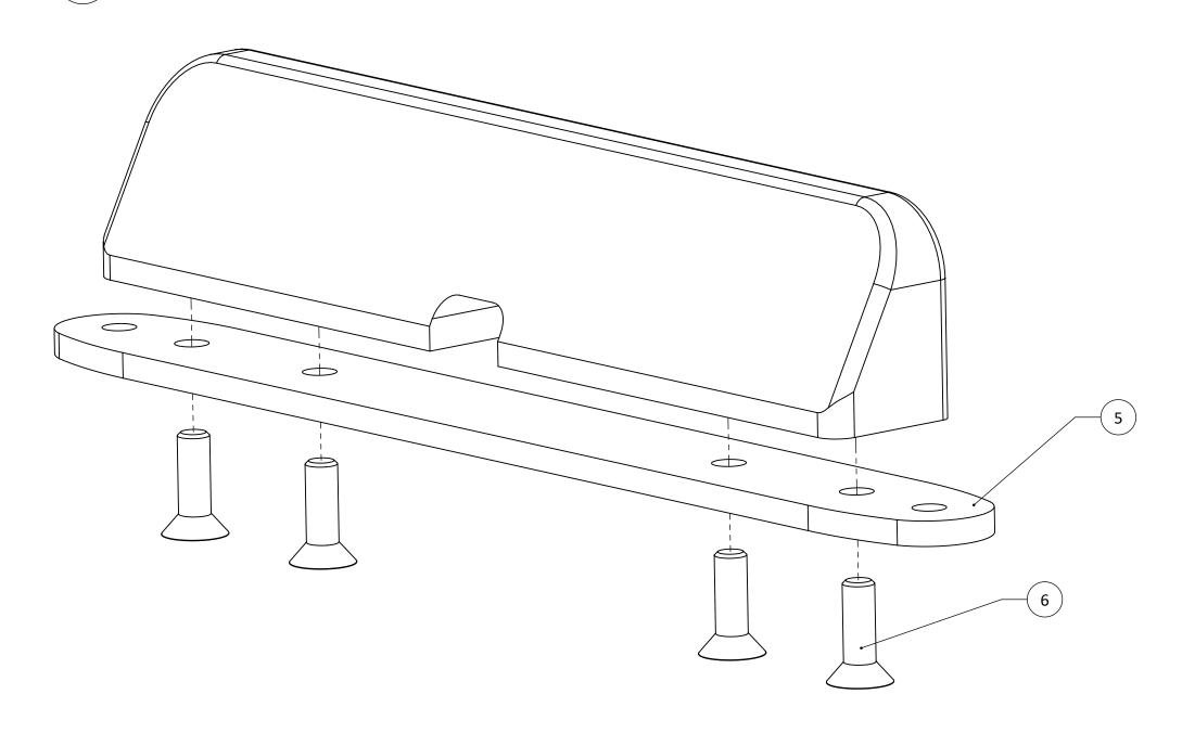
Determine desired mounting location. Use dimensions provided on page 2 to help with this process. Use one of the mounting plates, with the short end cap attached from previous step, to mark and drill holes. It is recommended that the angled surface of the short end cap faces forward.
