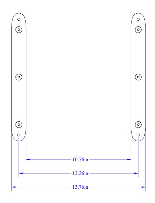
Attach one mounting plate (item 5 from BOM on page 1) to each end cap using the provided countersunk screws (item 6 ).
