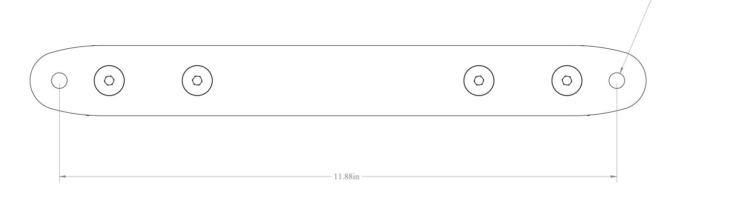
Using stainless washers (item 8), bolt the short end cap down using nyloc nuts (or similar). Due to varying mounting surface types and thicknesses, ensure the correct mounting bolts and hardware are used.
