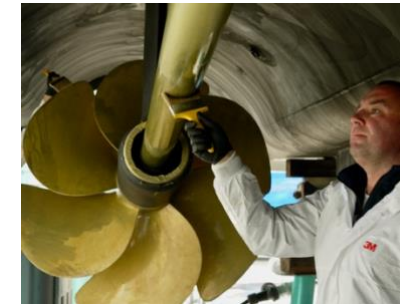
Clear Coat application
