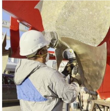
Surface preparation with grinder
