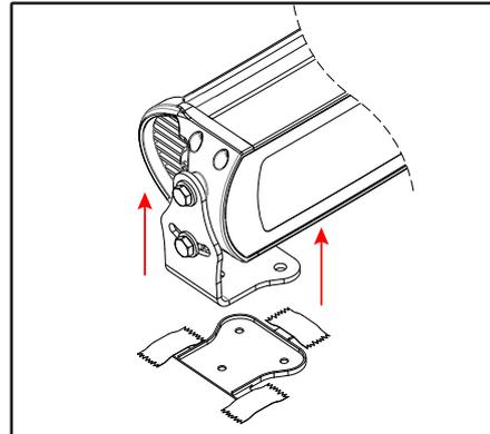
5. Use the bracket drill jig to drill a 4mm pilot hole followed by a final drill diameter of 6.5mm for the M6 mounting bolts.
