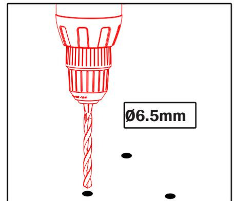
6. Remove brackets from light. Using the supplied fixing hardware fix the brackets to the boat. It is recommended that marine sealant (3M 4200) is used in and around the mounting holes. The spreader plate is required to go underneath the mounting surface and provides an even distribution of force when tightening. It is important to note that at this stage these mounting bolts are to be left loose as this is a crucial step in adjusting the angle of the light in the coming steps.
