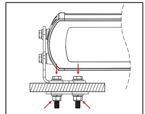
9. Locate a suitable entry point for the cable and drill a 9.5mm hole. The cable should always be in a 'fixed' position, no movement or rotation. The cable entry should be made watertight with marine sealant (3M 4200), the use of a cable gland is recommended.
