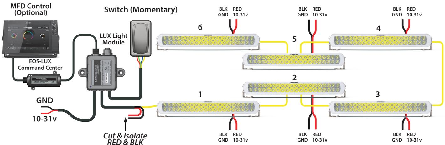
**Note :** *Black wire from each light and LUX Module should connect to common ground*
