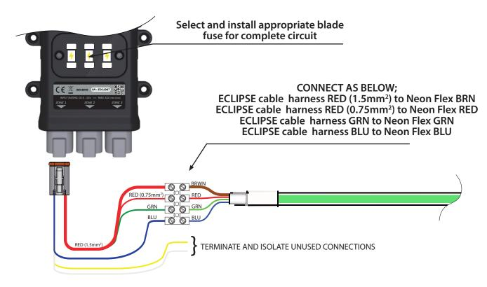
Note: Single color, dual color and RGB lights should not be added to the same zone output. Use a separate zone output for each type.
