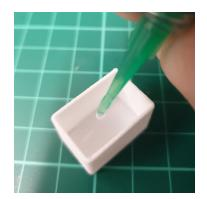
7. Fill the Blanking End Cap 1/3 of the way up with silicone adhesive (supplied).
