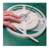
5. With the cut points on the outside, coil the Neon Flex back on to the reel so that the PCB is retracted back into the extrusion.
