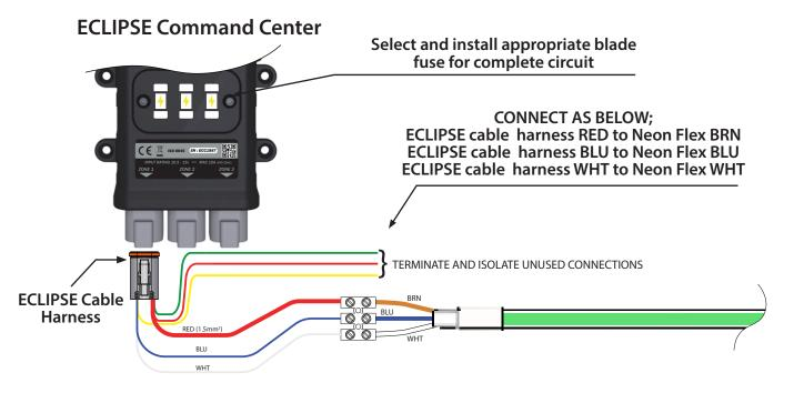
Note: Single color, dual color and RGB lights should not be added to the same zone output. Use a separate zone output for each type.
