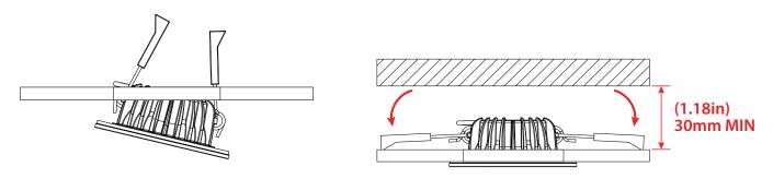
For exterior installations or wet areas it is recommended that the light is fixed in place using a suitable marine sealant / adhesive. *Remove the spring clips and the black gasket* from the fixture and dispense a small amount of adhesive around the glass bezel. Push into place using a slight rotation of the light to spread the adhesive evenly. Clean any excess adhesive using a soft cloth and soap and water – *DO NOT USE CHEMICAL CLEANERS*.
