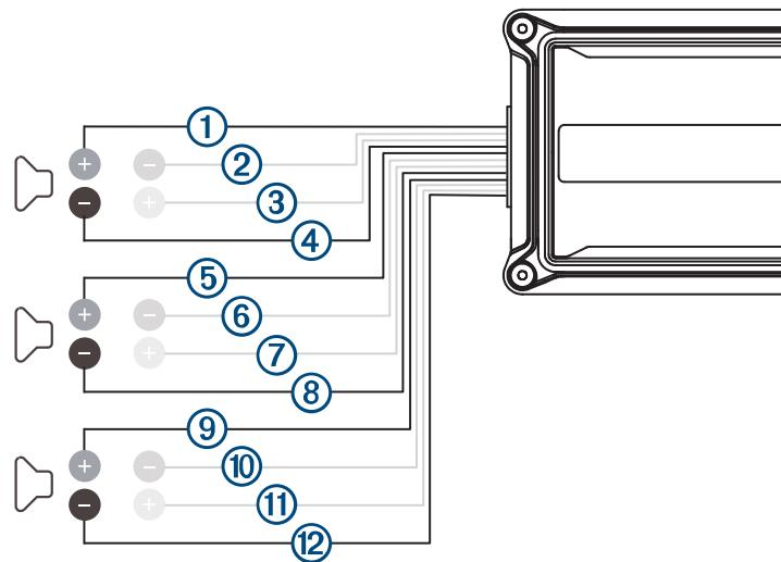
**Figure 4: Bridged Mode Outputs**
