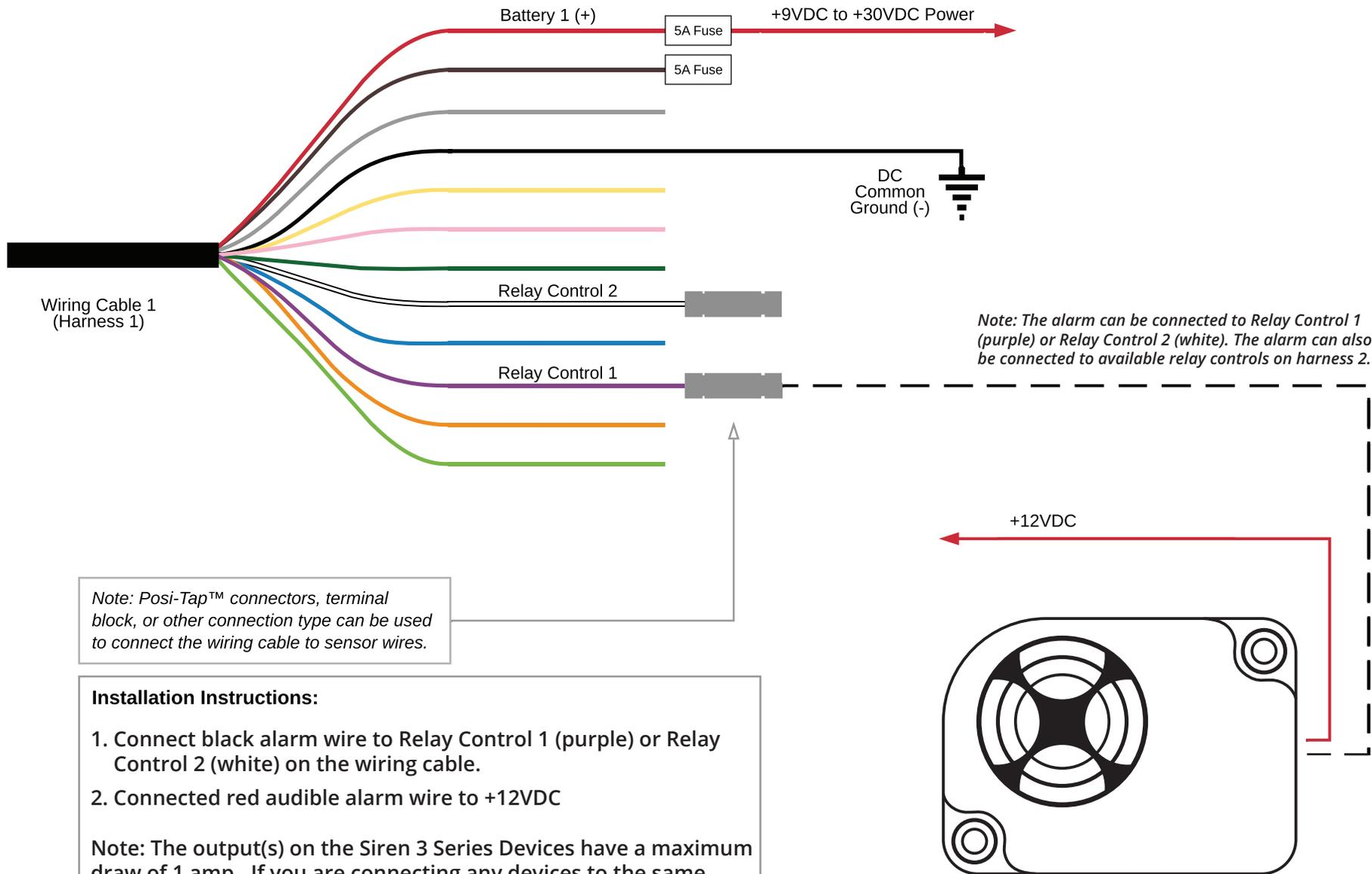
Note: Posi-Tap™ connectors, terminal block, or other connection type can be used to connect the wiring cable to sensor wires.
