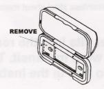
Slide the stereo through the front of the front cover. Follow the installation instructions in your stereo manual for attaching the stereo to the front cover. Usually this involves using mounting clamps or bending metal tabs on the stereo.
