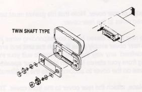
Attach front panel, mounting nuts, and knobs as per installation instructions of the stereo.
