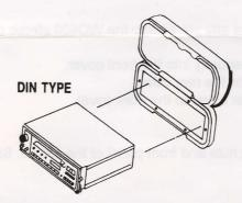
Place blue gasket over edge of rear cover. Note that his gasket must be between the front and rear covers before you attach the stereo wires to the rear cover.
