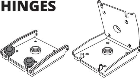
Seaview Hinge Adapters fold in any direction necessary for added height clearance.
