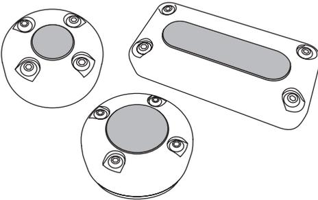
Seaview Cable Glands provide waterproof cable routing.
