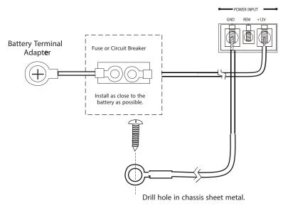
Make the ground lead as short as possible, leaving enough length to complete the installation. To ensure a good ground, scrape away any paint or undercoating to expose bare metal. Use a "ring" terminal of the proper gauge and an "outside star washer" (between the chassis and ring terminal) when making your ground connection.
