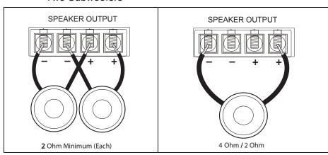
Minimum load is 1 Ohm for any combination of subwoofers
