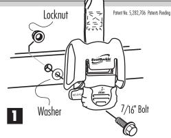
2. BoatBuckle should be mounted to trailer frame in such a position to enable the web to have as much of a straight line pull as possible. Web angle should not exceed a +/- 30 degree angle (forward or back) from vertical when in use, as shown.
