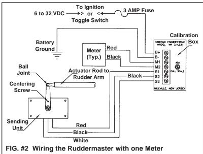
NOTE: Slight adjustment can be made by loosening set screw in the sender arm and rotating the sender shaft. It is important that the rudder arm and the sending unit arm continue to move parallel to each other hard over port to hard over starboard.
