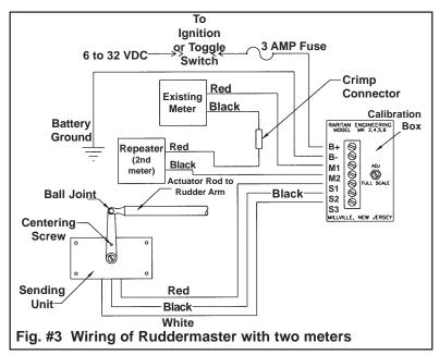
screw as far as it will go counter clockwise. The ohmmeter scale should indicate 0. Now turn the adjustment screw in a clockwise direction until it stops. The reading on the ohmmeter should show 50,000 (50K) ohms of resistance.
