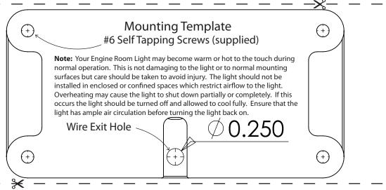
Thank you for purchasing the Engine Room Light. This light utilizes Lumitec's proprietary technology to cast a broad, even light over a wide area in a color optimized for easy viewing and reduced eye fatigue.
