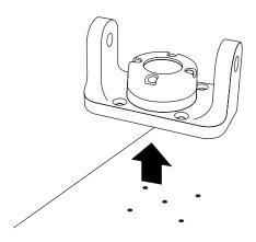
Drill out the four holes for mounting the adjustable base.
