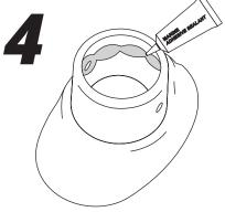
Apply marine adhesive sealant to the inside of the modular top where the pole will slide into. Be sure to get around the bolt holes.
