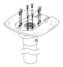
Apply marine adhesive sealant around the base of the modular top.
