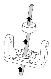
23 Secure the outer shell of the Cable Gland using the four screws.
