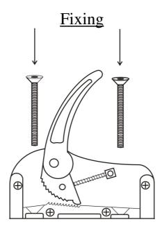
Use 6mm (1/4") Counter sunk stainless steel fastening, full nuts and penny washers to secure An Anti corrosive jointing compound is required between the counter sunk screws and the aluminium base of the clutch
