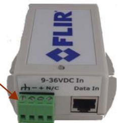
2. Attach vessel power to the green terminal block.
