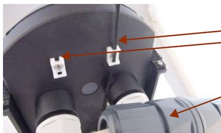
Thread zip tie through the two holes in the two anchors
