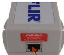
Insert Ethernet cable from the camera in this end
