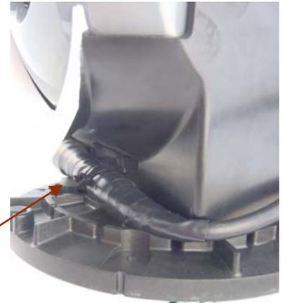
Front View: Sealed cable tied to camera base
