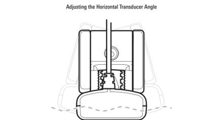
4. Once finalized, mark the correct position on the transom by tracing the silhouette of the transducer mounting bracket with a pencil or marker.
