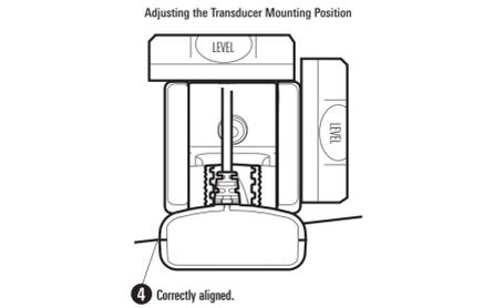
**Downward Slant:** The transducer has a natural downward slant of 4 to 5 degrees from leading edge to trailing edge. Looking at the back of the transducer, the seam should be slightly below the bottom of the hull.
