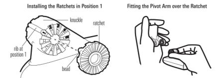
**NOTE:** The ratchets are keyed. Make sure that the square teeth on each ratchet face the square teeth on the transducer knuckle, and the triangular teeth face outward.
