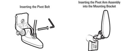
**NOTE:** If the pivot assembly is snapped closed over the mounting bracket, use a flat head screwdriver or similar tool to gently pry the assembly away from the mounting bracket.
