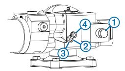
**3** Remove the mounting pin ④ to release the drive unit from the base.
