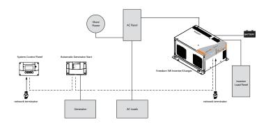
Figure 2 Typical Xanbus System Diagram
