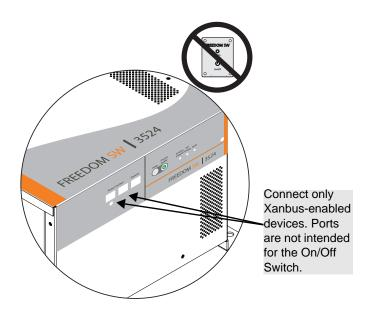
Figure 14 Connecting to a Xanbus Network Port
