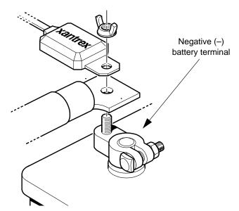
Figure 11 BTS Mounted on the Negative Battery Terminal
