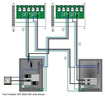
Figure 16 Parallel Stacking Using Two Freedom SW 3524-230s
