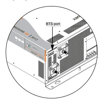
Figure 12 Connecting the BTS Cable to BTS Port
