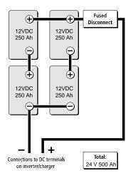
Figure 21 Batteries in Series-Parallel Connections
