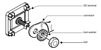
Figure 7 DC Cable Connections
