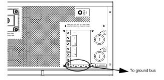
Figure 6 AC Wiring Compartment
