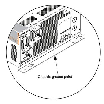
Figure 9 DC Wiring and DC Grounding
