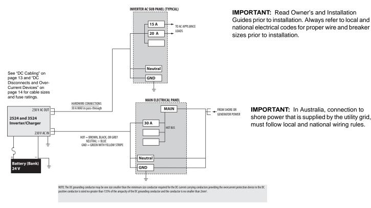
Figure 4 Wiring and Breakers Block Diagram for Freedom SW 230V 2524 / 3524
