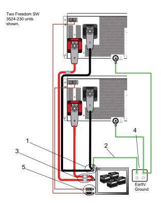
Figure 17 Connecting Battery Cables and DC Earth/Ground Wires
