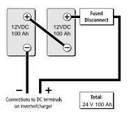
Figure 20 Batteries Connected in Series
