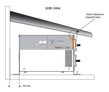
Figure 22 Drip Shield Placement (Desktop Mount)
