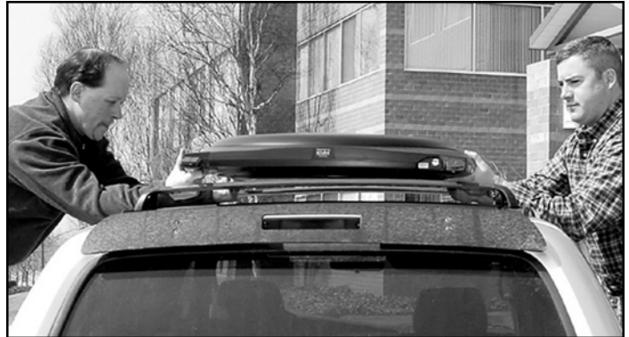
Figure 6: Placing the Antenna on the Crossbars
