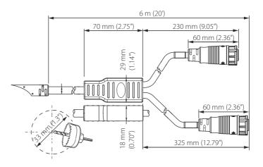
A 33mm (1.3") diameter hole is recommended for cable clearance.
