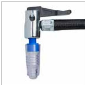
**STEP 2 -** If you are using a gas station or portable air compressor, set your gauge at 2 PSI. Do not go beyond this setting. Insert the inflation adapter in the valve opening and apply the nozzle to the adapter and depress to start the air flowing.
