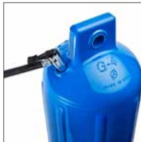
**STEP 3 -** Fill the Polyform fender or buoy until the walls are fully expanded. The best way to check that is to measure the circumference of the particular product and match the chart measurement. You should also be able to easily push with your thumb and depress the wall 1/4 inch.
