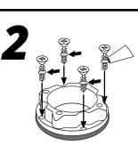
Drill pilot holes and secure the base. Apply marine sealant to the threads of the screws.
