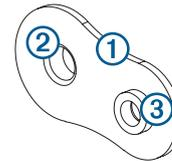
If you are using a nut plate, the smaller hole ③ on the nut plate should line up with the smaller hole on the template.
