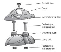
Note: When mounting lamp units side by side allow a gap of 5mm to ensure screw cap removal.
