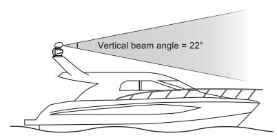
It is rarely possible to place the antenna unit where a completely clear view in all
