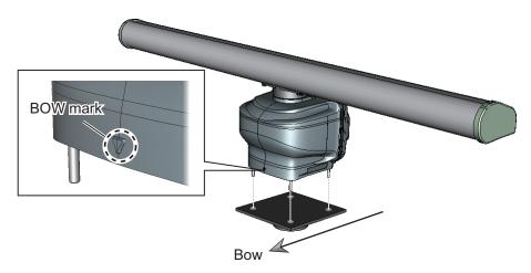
7. Secure the antenna unit, using the supplied flat washers (M12, 4 pcs), spring washers (M12, 4 pcs), and hex. nuts (M12, 8 pcs).
