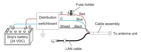
**Note 1:** The antenna unit has no power switch. Connect the antenna unit to a distribution switchboard with a switch for power control.
