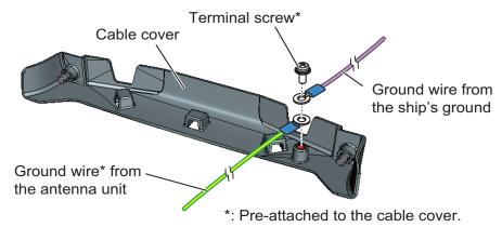
5. Apply silicone rubber to the ground terminal after fastening the terminal screw.
