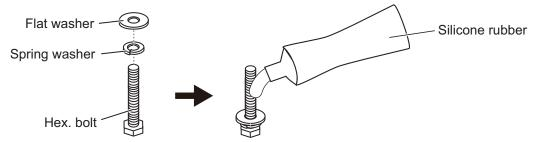
6. Fasten the radiator to the radiator bracket, using four bolt assemblies prepared at step 5.
