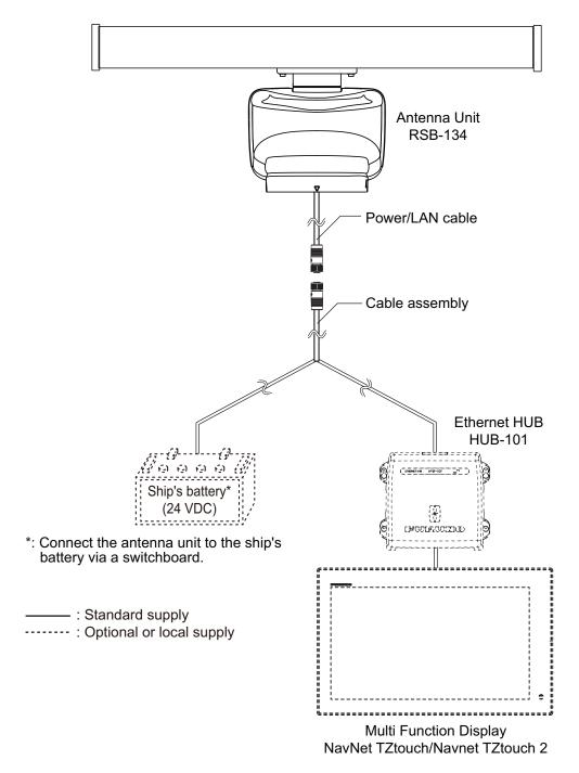
This radar series is compatible with the FURUNO Multi Function Displays and software version combinations shown below. The combination with other models may not operate properly.
