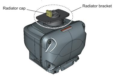
2. Apply silicone rubber to the surface of the radiator bracket as shown in the figure below.
