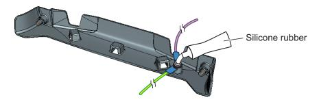
6. Secure the ground wire to the ship's ground.
