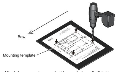
2. Attach four corrosion-proof rubber pads (supplied) to the mounting holes.
