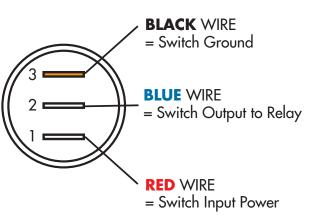
WIRING DIAGRAM FOR NON-RELAY HARNESS
