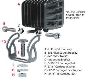
**MOUNT INSTRUCTIONS & DIAGRAM FOR SR-Q SERIES** 1. Place 5/16"- 18 Carriage Bolt (E) into Mounting Bracket (D).
