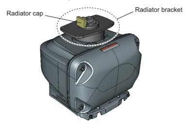
2. Apply marine sealant to the surface of the radiator bracket as shown in the figure below.
