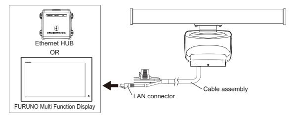
**Note 2:** When LAN cable extension is needed, use the optional LAN cable (MOD-Z072) and joint box (TL-CAT-012). After connection is completed, wrap the connector with vinyl tape to waterproof the LAN connector.
