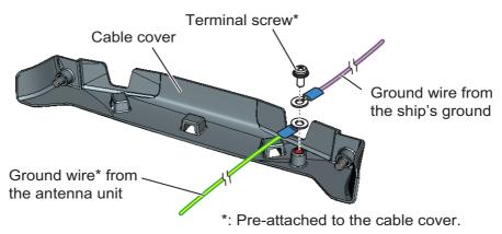
5. Apply marine sealant to the ground terminal after fastening the terminal screw.
