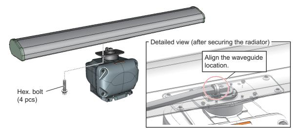
Apply marine sealant to the holes and bolts at the locations indicated with arrows in the figure below. Also apply marine sealant to the junction between the radiator and the radiator bracket.
