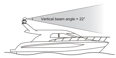
• It is rarely possible to place the antenna unit where a completely clear view in all directions is available. After fitting the antenna, determining any shadow sectors, their angle and bearing, and their influence on the radar is recommended.
