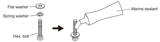
6. Fasten the radiator to the radiator bracket, using the four bolt assemblies prepared at step 5.
