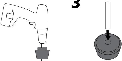
Apply small amount of soapy water to the tube and slowly drill the rubber plug.
