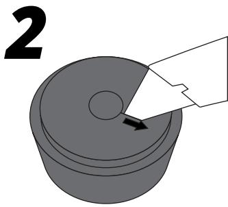
Using a sharp razor blade or knife, cut the rubber grommet from the cable hole outward.
