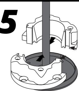
Combine the two halves of the plastic base and mount onto rubber base gasket. Be sure to stagger the seams as shown by the two black arrows.
