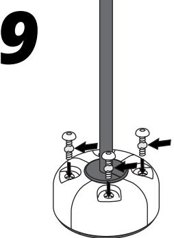
Apply marine sealant to the four allen head screws and tighten.
