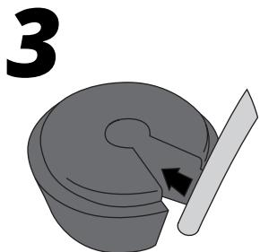
Wrap the rubber grommet around the electronic cable.
