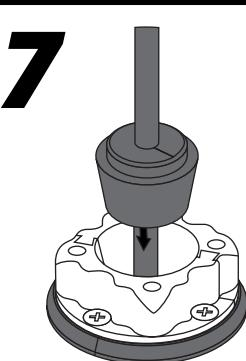
Slide the rubber plug down into the plastic base.
