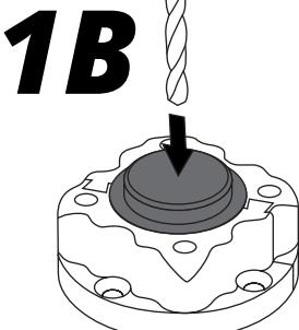
If using a drill bit, the drill should be run repeatedly through the rubber.
