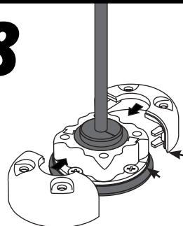
Combine the two halves of the outer shell. These will snap together with a click. Be sure to stagger the seams as shown by the two black arrows.
