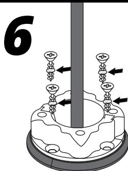
Secure the base to the mounting surface with the four screws. Apply marine sealant to the threads.
