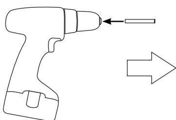
Insert drill tube into drill motor, and leave enough length to get through the tapered plug.
