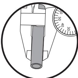
Measure your cable diameter and select the appropriate drill tube provided. Cable diameter +.01/-03
