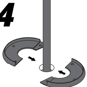
Apply the rubber base gasket to the mounting surface.
