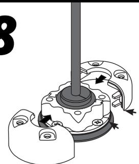
Combine the two halves of the outer shell. These will snap together with a click. Be sure to stagger the seams as shown by the two black arrows.
