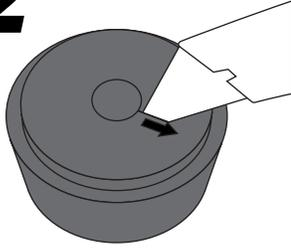
Using a sharp razor blade or knife, cut the rubber grommet from the cable hole outward.
