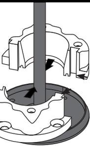
Combine the two halves of the plastic base and mount onto rubber base gasket. Be sure to stagger the seams as shown by the two black arrows.
