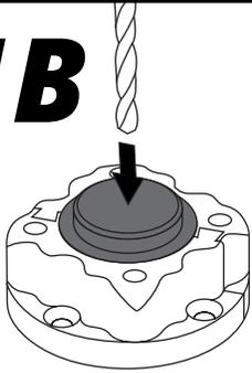
If using a drill bit, the drill should be run repeatedly through the rubber.
