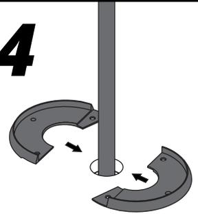
Apply the rubber base gasket to the mounting surface.
