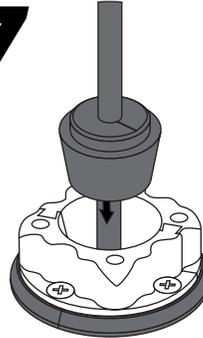
Slide the rubber plug down into the plastic base.
