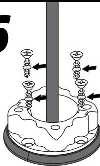
Secure the base to the mounting surface with the four screws. Apply marine sealant to the threads.
