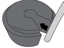
Wrap the rubber grommet around the electronic cable.
