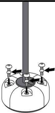
Apply marine sealant to the four allen head screws and tighten.
