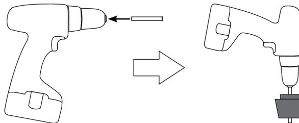
Insert drill tube into drill motor, and leave enough length to get through the tapered plug.
