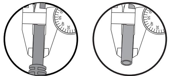
Measure your cable diameter and select the appropriate drill tube provided. Cable diameter  $+0.01/-0.03$
