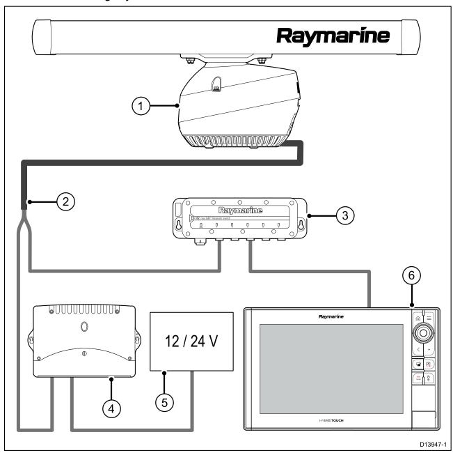
**Note:** Some power connections are omitted from this illustration. The network switch and multifunction display each require a dedicated power connection.
