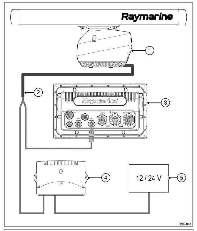
**Note:** Some power connections are omitted from this illustration. The network switch and multifunction display each require a dedicated power connection.
