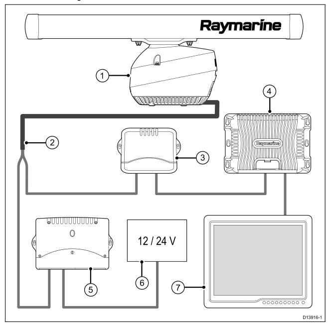
**Note:** Some power connections are omitted from this illustration. The network switch, processor, and display each require a dedicated power connection.
