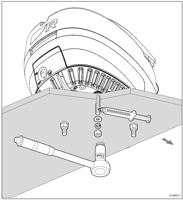
12. Ensure all 4 sets of nuts and washers are used to secure the pedestal to the mounting platform. There should be no more than 6 mm of excess stud below the nut. Cut-off any excess stud.
