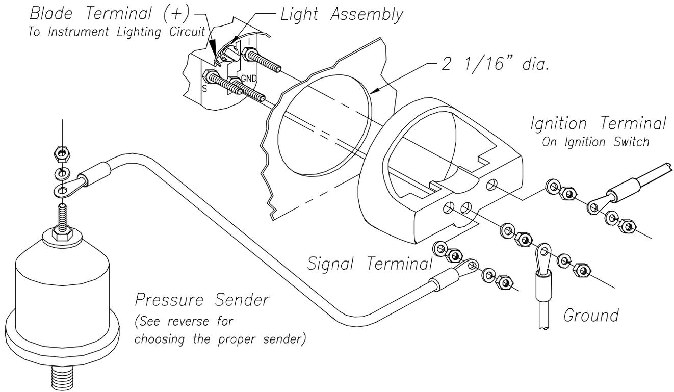
**CAUTION:** Disconnect the battery during installation. Tighten nuts on the backclamp only slightly more than you can tighten with your fingers. Six **inch-pounds** of torque is sufficient. Over tightening may result in damage to the instrument and may void your warranty.
