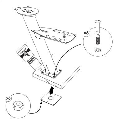
Attach the marine electronics to the Dual Mount. Use the remaining four nylon shoulder washers with marine adhesive sealant when securing the closed dome radar.
