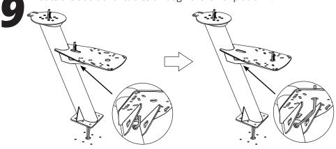
Apply to marine adhesive sealant to the base of the mount.
