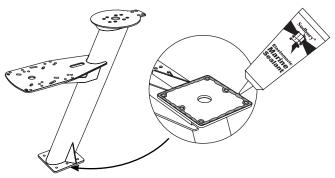
Place the Dual Mount onto the mounting surface.
