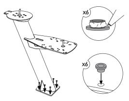
Use the provided backing plate and your own hardware to secure the Dual Mount. Apply marine adhesive sealant to all bolt holes.
