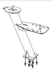
Apply marine adhesive sealant to the six nylon shoulder washers and insert them into the base.
