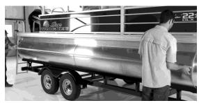
Measure the length of the pontoon tube. If the PontoonGuard is too long, trim the PontoonGuard with a utility knife on the rear squared edge for a precise fit.
