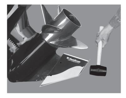
**STEP 1**. Ensure proper fit before installing the Megaware SkegGuard<sup>™</sup>. There must be at least two to three inches of upper skeg remaining to secure the new Megaware SkegGuard<sup>™</sup> to. If any portion of the skeg has been bent or distorted, fitment may be difficult without re-conforming to original shape.
