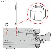
While holding (H) nuts in place, attach ball adapter to back of holder using (G) screws. RAM® logo must be facing in the shown direction. Attach additional (L) screws.
