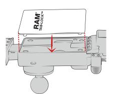
Secure using (J) screws on back of slide assembly. Lock must be engaged to access all four holes as shown.
