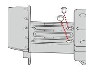
Attach (M) screws from behind the 9 internal slide. Do not fully tighten (slides must remain loose).
