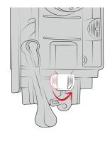
Insert top slide over internal vehicle dock.
