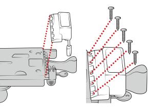
Using (K) screws, attach top docking cup to top slide with numbers facing down.
