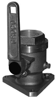
**Lubrication:** BV seacocks are fitted with one drain plug and one zerk fitting. The zerk serves as an additional drain plug but also provides for the injection of GROCO U-LUBE lubricant into the space between the ball and the valve body. U-LUBE (available in 3-oz or 14-oz tubes) is specially formulated for ball valves to lubricate wear parts and to discourage the accumulation of nuisance marine growth.
