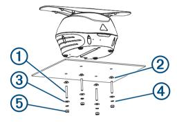
To avoid damaging the pedestal, you should stop tightening the threaded rods when they no longer turn easily.
